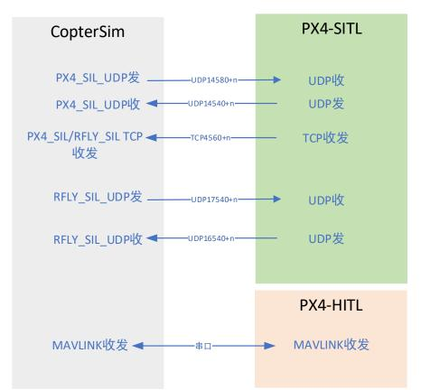
At the same time, the messages sent by CopterSim to PX4 via TCP include HIL\_GPS, HIL\_S ENSOR, RC\_CHANNELS\_OVERRIDE. HIL\_GPS is the simulated GPS data, and HIL\_SENSOR simulates the IMU data, including the data of gyroscope, accelerometer, magnetometer, barometer. And RC\_CHANNELS\_OVERRIDE is the simulation of the remote control data.
